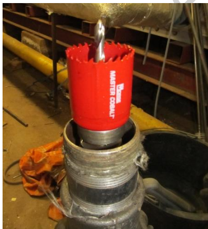
Above: A pilot bit and hole cutter (44mm) installed onto the drilling shaft.
