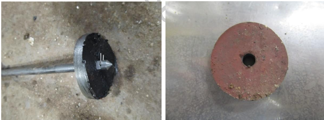
Above: the coupon has been caught by the catcher assembly, and removed ready to hand to client for inspection.
